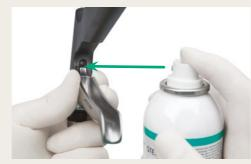
Lubricate the defined places on the clip applier with AESCULAP® Sterilit® Oil after each cleaning cycle.
